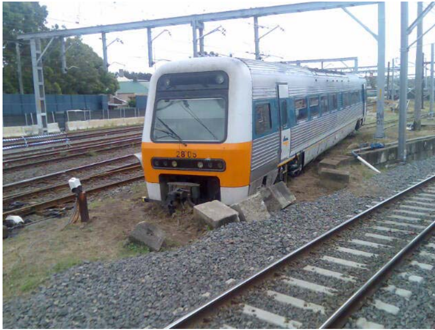
A brake failure put Endeavour power car 2805 in the dirt at Eveleigh. The Up Eastern suburbs line is in the foreground while the Down Illawarra mainline is directly behind the Endeavour. November 4th, 2006. Photo: James Percival
