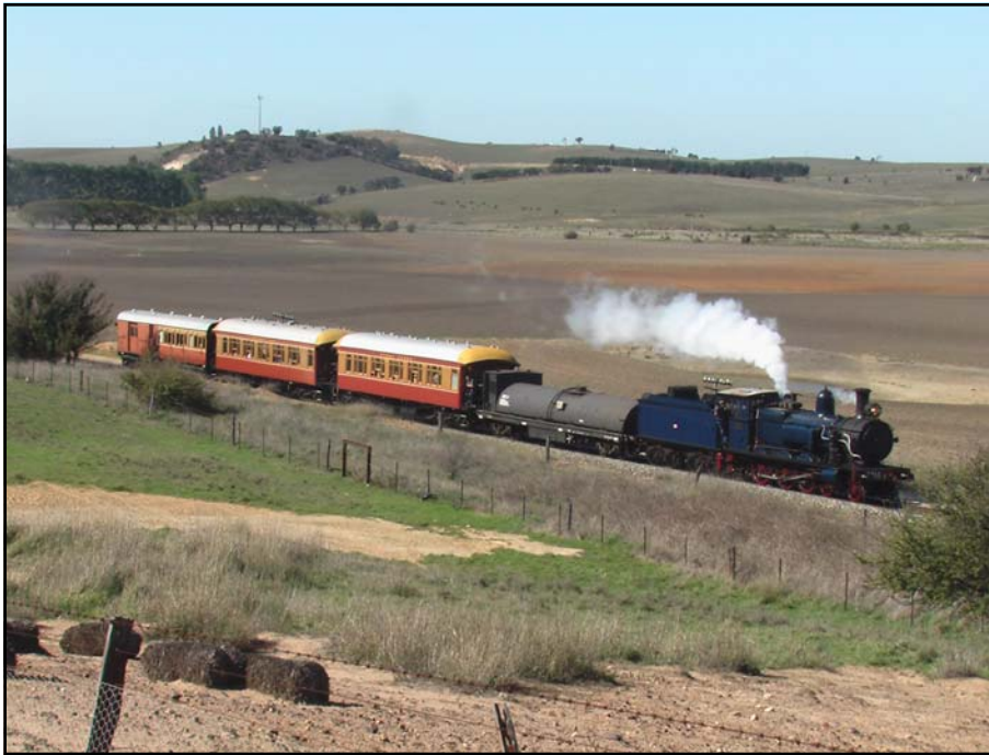
3016 marches up the hill just south of Tarago on the Canberra line. Built as a suburban tank engine, 3016 was converted to a light tender engine for use on the many light branch lines around NSW. A later conversion saw it fitted with a superheated boiler. April 1, 2007. Photo: Glenn Percival
