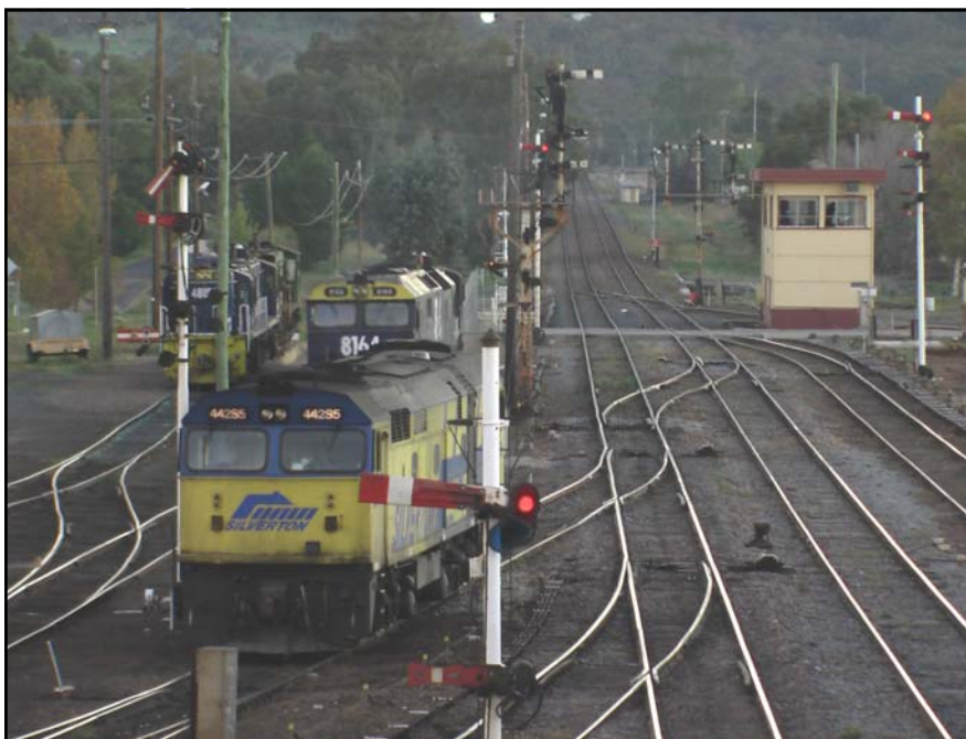
ARTC's extensive resignalling work along the Main South will shortly see the end of scenes such as this. A forest of mechanically operated lower quadrant semaphore signals surround Silverton's 442S5 as it shunts in Cootamundra yard. Cootamundra South Box, which controls these signals, is in the background. May 11, 2007. Photo: Glenn Percival
