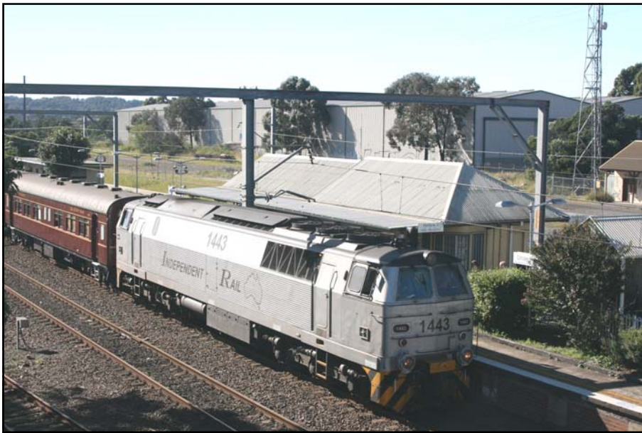
Independent Rail MZ class diesel 1443 heads 3801 limited's 'Cockatoo Run' on a trip to Kiama. 10 MZ class were imported from Denmark and mostly see use on Independent Rail's freight trains. May 20, 2007. Photo: Mic Wade
